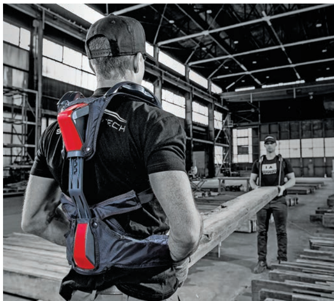
The StrongArm Technologies Ergo-Skeleton is an external spine that attaches to the worker's back and improves lifting dynamics, safety and efficiency.
