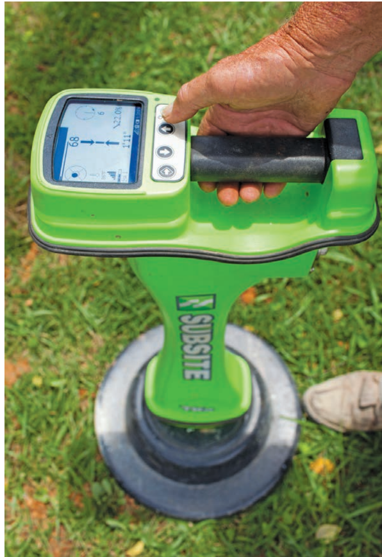
Poor ground connections or bad ground placement are two of the most common rookie errors in utility locating. Incorrect frequency selection — starting on the high end, for example — is another common mistake.
