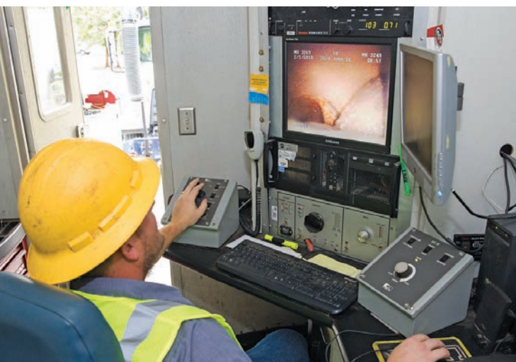
Will Giebel operates a CUES camera controller with POSM video software while inspecting a sewer line.
