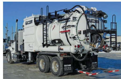
Guzzler CL dense phase off-load option
