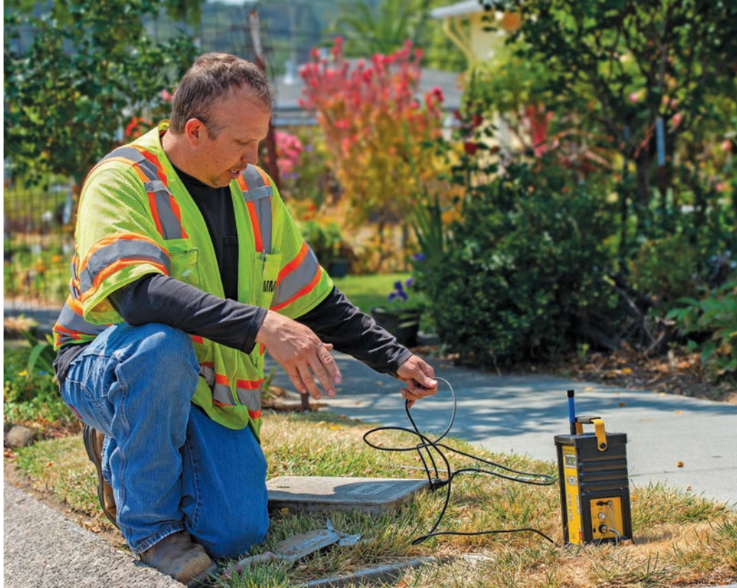
Kevin Barkdull sets up equipment to listen for leaks at a valve pit.
