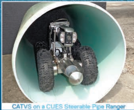
CATVS on a CUES Steerable Pipe Ranger
