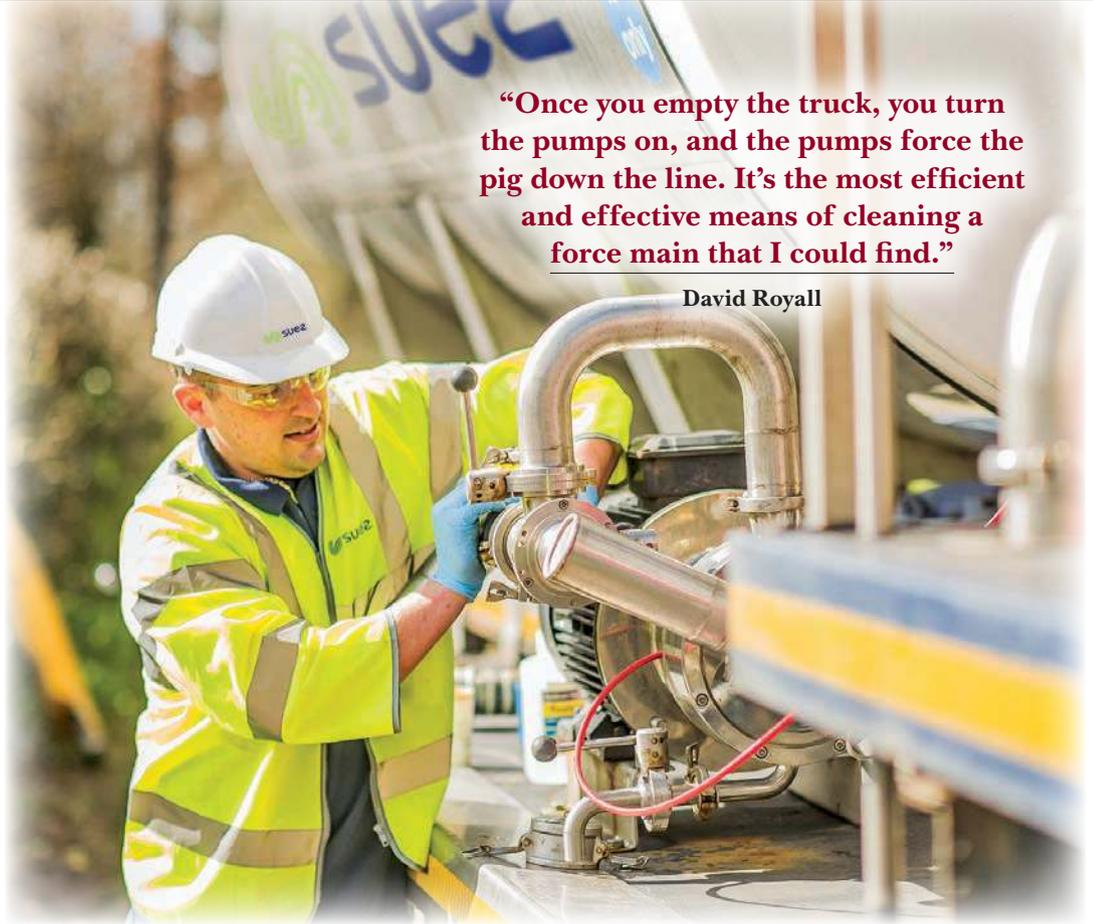
**“Once you empty the truck, you turn the pumps on, and the pumps force the pig down the line. It’s the most efficient and effective means of cleaning a force main that I could find.”**
