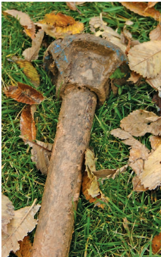
Acidic soil can rapidly corrode cast iron infrastructure and compromise the entire curb box/curb stop apparatus.
