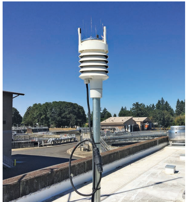
The water reclamation facility in Albany, Oregon, uses an Orion Weather Station all-in-one sensor from Columbia Weather Systems to monitor wind speed and direction with ultrasonic technology, as well as rainfall, temperature, humidity and barometric pressure.
