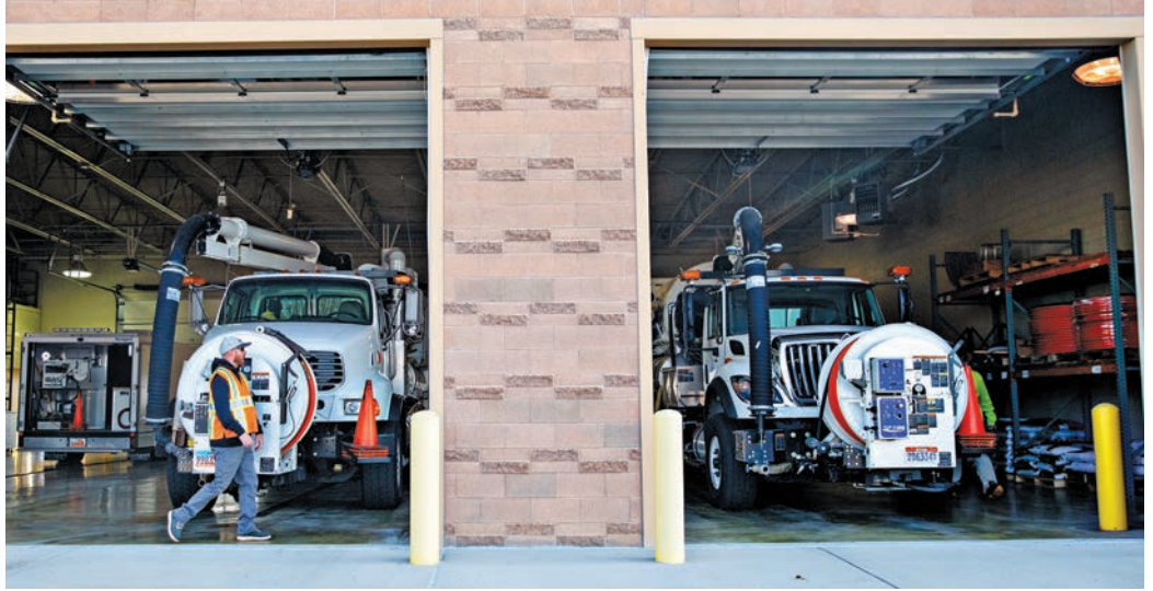
Corey Hudson, a linesman at Sandy Suburban Improvement District, checks over a Vactor combo truck before heading out to clean sewer lines.
