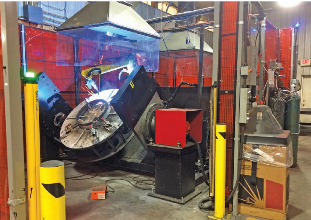
In addition to its products, American Highway Products designs the machines that make the products, like this robotic welder. The company's jobshop manufacturing approach allows it to make exactly what its customers need based on their dimensions.
