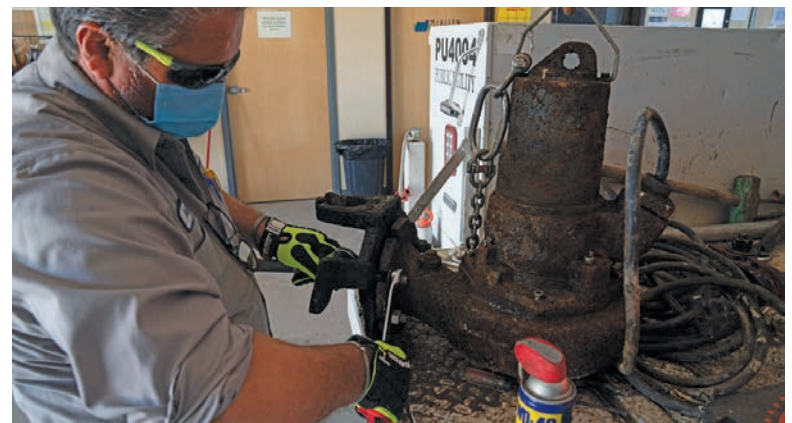
Mechanic Miguel A. Treviño fixes the impeller from an ABS pump at the South Wastewater Treatment Plant in McAllen, Texas.
