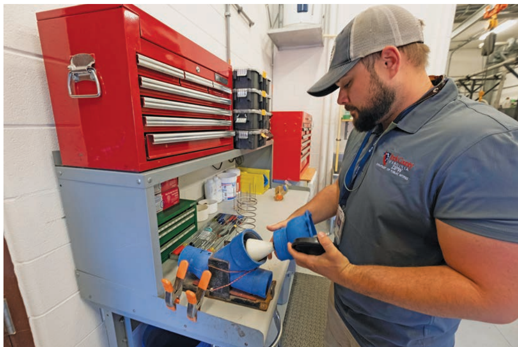
Top: Charles Meredith rebuilds a residential check valve for a vacuum system pit.
