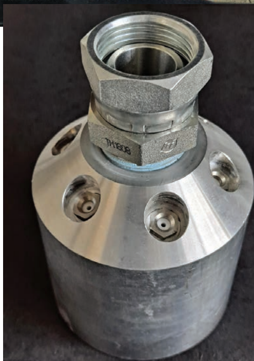
Jet angles, orifice size and cohesive flow play an important role in nozzle efficiency. (Photos courtesy of NCPI)
