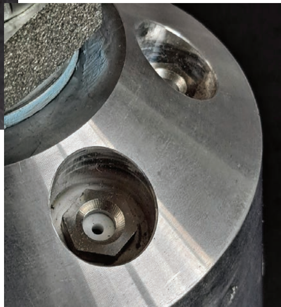
Jet angles, orifice size and cohesive flow play an important role in nozzle efficiency. (Photos courtesy of NCPI)
