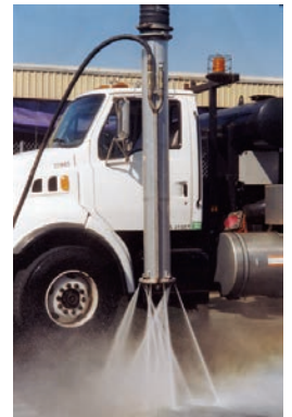
Soil Surgeon hydroexcavating tool
