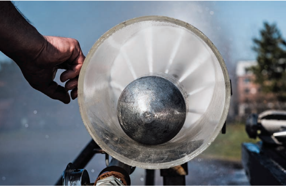
The most efficient nozzles offer tight water patterns that effectively clean the pipe wall and create a powerful water stream to move debris long distances and propel the nozzle.
