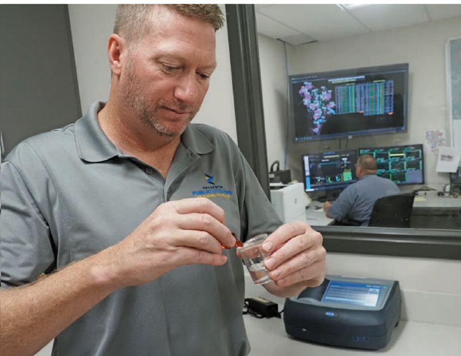
RPU Environmental Regulations Affairs Coordinator Todd Osweiler conducts a fluoride test on a Rochester public water sample in the city's water lab. Behind him is the water department control room.
