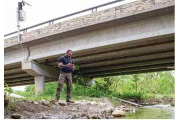
Brandon Smith, Frisco stormwater maintenance supervisor, checks stream gauge data through the online portal using his smartphone. The system allows for 24/7 access to review stream stage levels and water quality parameters.
