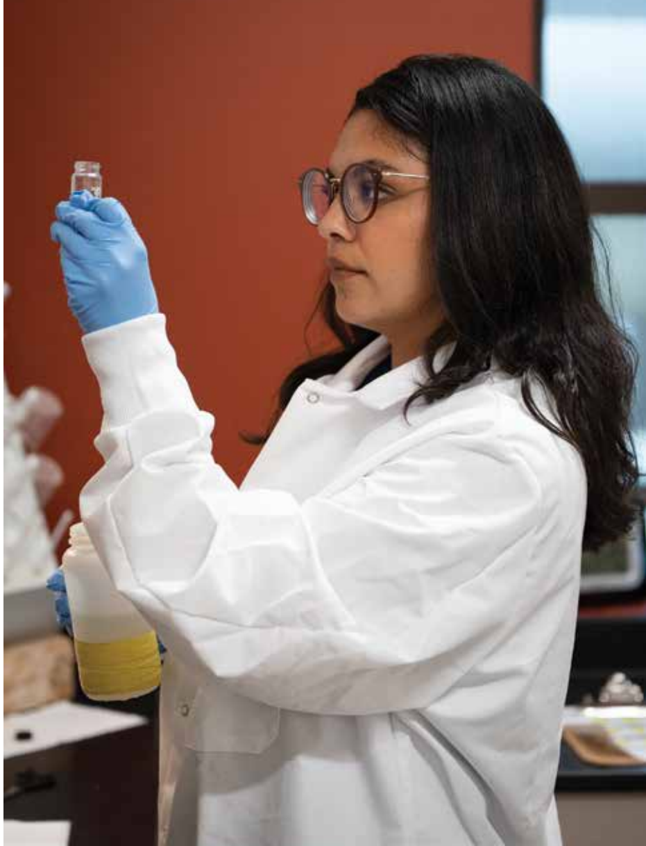
Krystal Accuosti tests a water sample to make sure it's compatible with the five other water supplies that will potentially mix with Vista Ridge water in the SAWS water distribution system.
