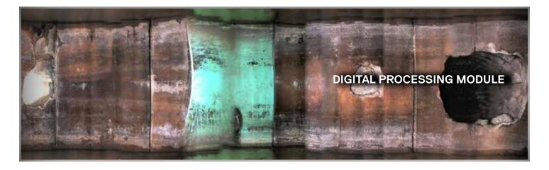
Video is stitched via the CUES GraniteNet software digital processing module. Flat images are available immediately following the inspection while LIVE video is available during/throughout the inspection. Virtual pan, tilt, and zoom plus a flat unfolded view of the entire surveyed pipe, enables rapid condition assessment review, significantly faster than traditional video inspection review. An expanded flat view is provided for additional detail with measuring capabilities.
