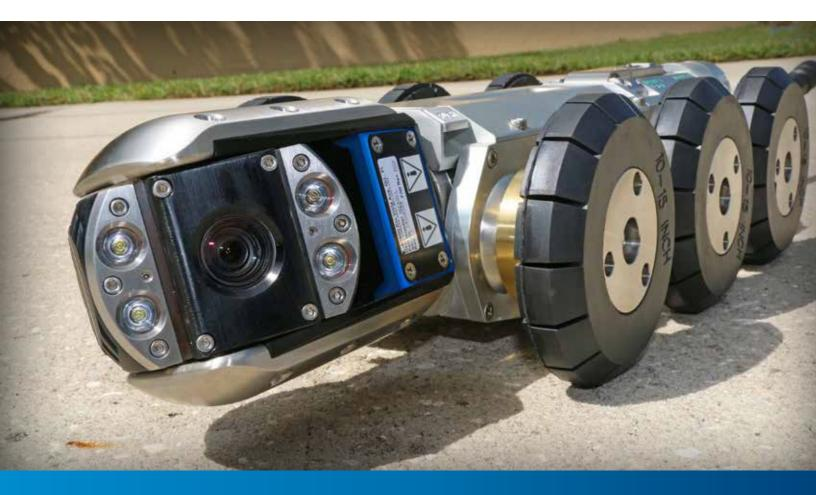
The OZIII-S camera provides up to 120:1 optical/ digital zoom, automatic focus, as well as remote focus and iris control, to assure the best quality video within varying pipe conditions. The OZIII-S optical zoom pan-and-tilt camera offers built-in directional field-replaceable lighting for 6"-72" (152 -1829 mm) pipe to produce the highest quality image details of your CCTV pipeline inspection.
