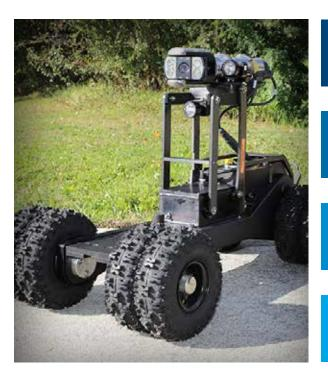
SMM is a self-propelled power forward, power reverse, and freewheel multiconductor transporter.
