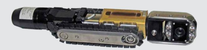
Ultra Shorty III features a reduced camera/tractor length with the CUES OZIII Camera to facilitate line entry through inverts with limited space and traverses 22, 45, and 90 degree sweeps in smaller diameter lines. The transporter includes weighted adapter blocks to optically center the camera and a built-in connector and protective housing for direct insertion of the OZIII camera; no camera interface cables are required.
