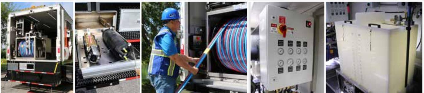
Applications include pipe stabilization and support, joint testing and sealing of mainline and lateral joints, manholes, junction boxes, large diameter pipes, or any other low pressure waterproofing application. All systems can be configured to run Urethane, Acrylamide and Acrylate grouts. Dry freight box (for export), trailer-mounted systems, and retrofits are also available. Combo trucks are available for TV, Cutter, & Easy Grout.
