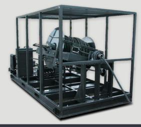
NLB's high-capacity hydraulicallydriven Roto-Reel® hose reel spools a hose at 60 feet per minute and feeds it out at 40 feet per minute.
