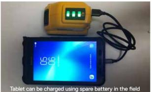
ablet can be charged using spare battery in the field with optional DeWalt® USB adapter
