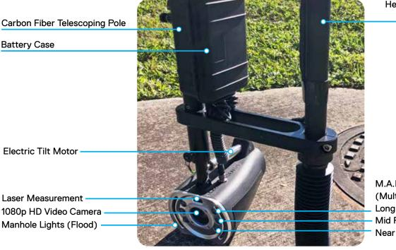
M.A.P. Lighting (Multiple Aspheric Projection) Long Range LED's (2) Mid Range LED's (2) Near Range LED's (2)
